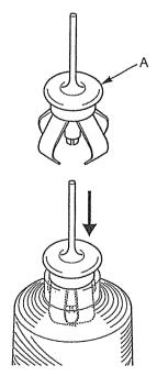
2. Pass the thread toward the top from the inside of B set. And cover the A set with the B set. After that, do the setting of thread in the machine as usual.
